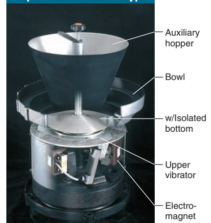
Exploded view of N25 type
